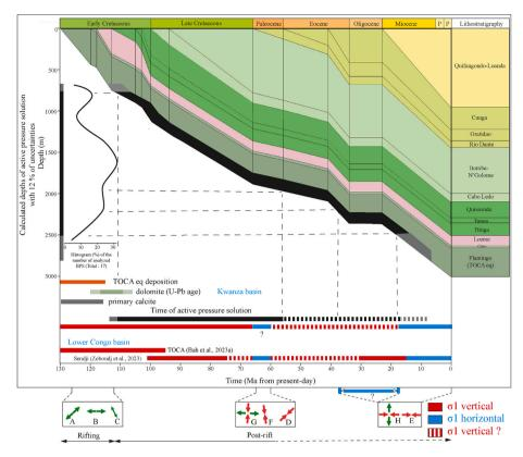
Fig. 10. Burial model constructed from Well-4. The depth on the model is counted from the sea-bed. The calculated depth range of active pressure-solution from bedding-parallel stylolite inversion is reported for the TOCA eq in black on the y-axis, while grey corresponds to uncertainty. The stress regimes revealed by inversion of calcite twins are also reported (map view).
