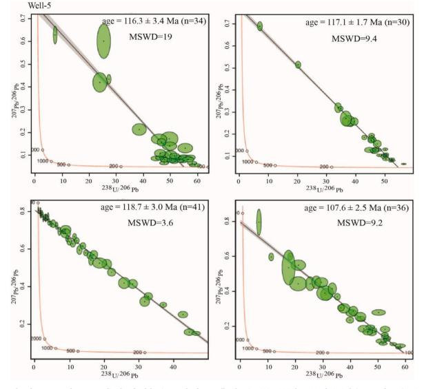
Fig. 8. Examples of Tera–Wasserburg concordia plots for dolomite samples from Well-5 showing 238U/206 Pb vs. 207Pb/206 Pb (n – no. of spots). MSWD – mean square of weighted deviates.
