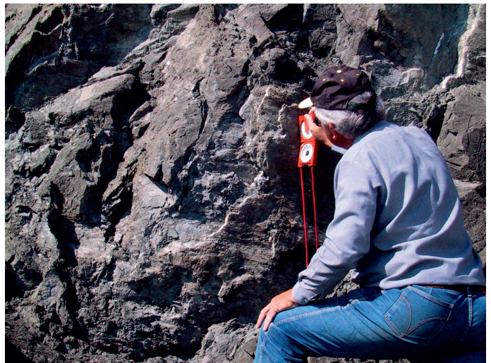
PHOTO 4. – Jacques measuring a right-lateral strike-slip fault in a Permian dyke, S. Sandby quarry, Scania Sweden, 2005.
