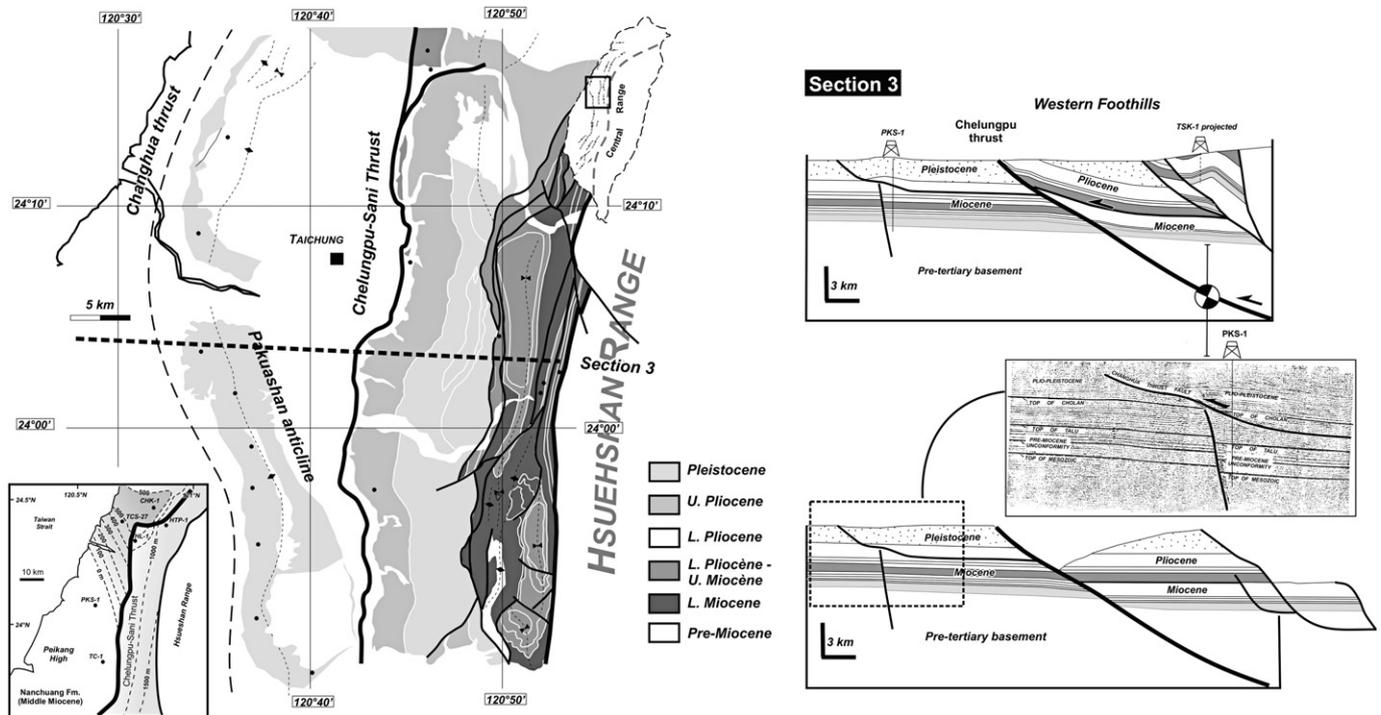
Fig. 7. Structural map of the northern-central part of the Western Foothills (Taichung area) and a balanced/restored section. An example of a seismic reflection profile across the Pakuashan anticline is shown (Chen, 1978). Insert: Isopachs map of the Nanchuang formation (Middle Miocene) from (Chou, 1980). These isopachs together with the depth of the Chichi earthquake ( $12 \pm 5$  km) suggest that the thrust may be related to the inversion of an inherited basement normal fault.
