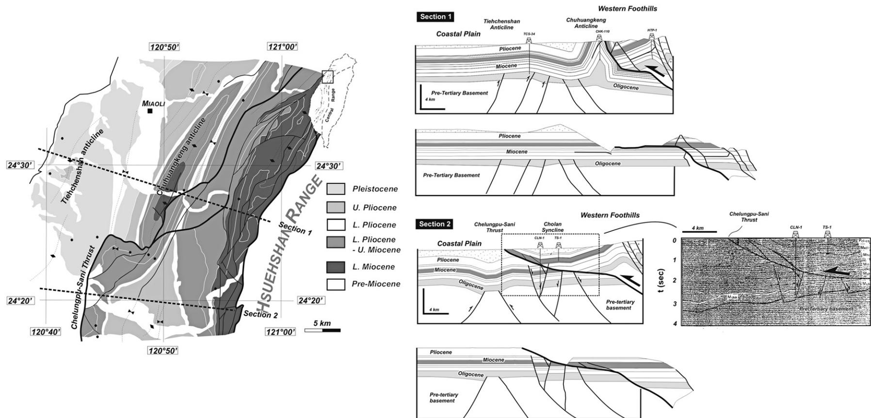
Fig. 5. Structural map of the northern Western Foothills (Miaoli area) and balanced/restored sections across the Miaoli area. An example of a seismic profile used to constrain our cross-sections is shown after (Hung and Wiltschko, 1993). Black dots correspond to locations of new sites where fault slip data have been collected and paleostress tensors computed.
