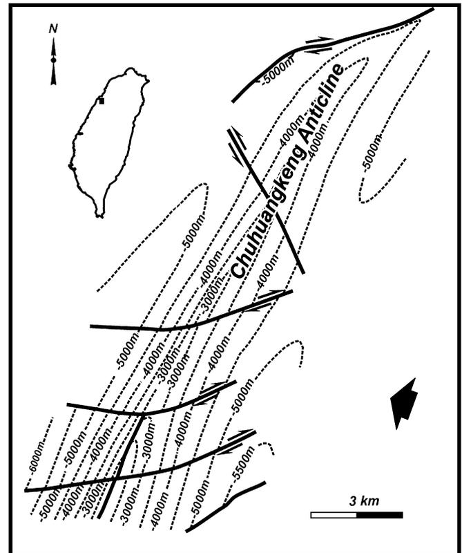
Fig. 6. Isobaths of the top of the Mushan Formation (Upper Oligocene) in the Chuhuangkeng anticline (Wey et al., 1992). This figure outlines the occurrence of inherited normal faults reactivated as transpressional dextral strike-slip faults (consistent with an average  $N110^\circ$  compression).
