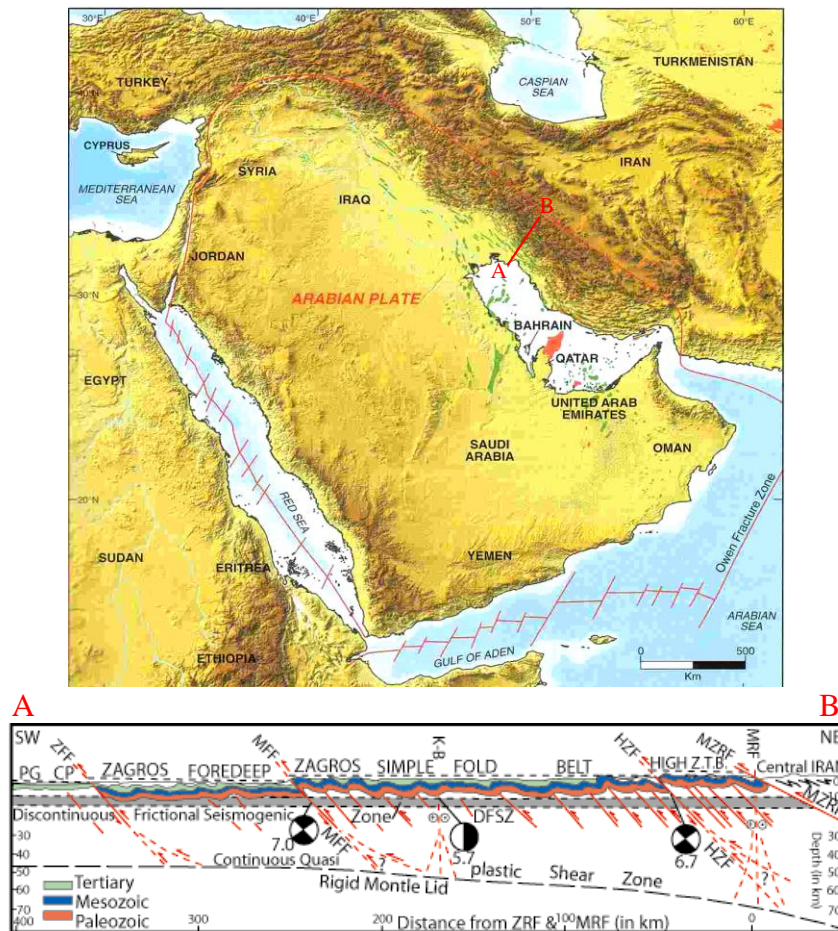
Fig. III.13: Topographic map showing the position of the Zagros folds belt between Arabian plate and central Iran (dark brown color). Down: Simplified transverse cross section of the Zagros active fold-thrust mountain belt. (Falcon, 1974; Hubber, 1977; Berberian, 1995) Abbreviations used: CP = Coastal plain; DFSZ = discontinuous- frictional-seismogenic zone; High Z.T.B = High Zagros Thrust Belt; HZF = High Zagros Fault; K-B = Kazerun-Borazjan active right lateral strike-slip fault; MFF = Mountain Front Fault; MRF = Main Recent active fault; PG = Persian Gulf; ZFF = Zagros Foredeep fault.
