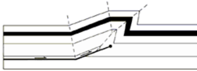
Fig.I.12: Fault-propagation fold ; layers in advance of propagating fault tip are folded.
