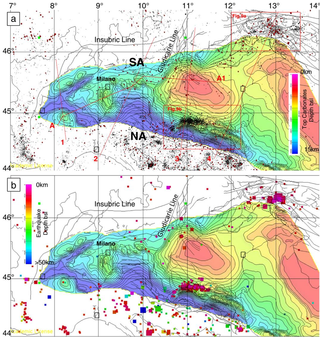
**Fig. 5.** Po Valley top Mesozoic Carbonates 3D grid by contouring and depth colouring, earthquakes and tectonics: map view; a) structures against all instrumental and historical earthquakes. Location of sections and selected domains in Figs. 7, 8, and 9 is indicated; b) structures against instrumental earthquakes ( $4 < M < 7$ ) coloured by depth. Horizontal net dimension is 80 km. Latitude and longitude values are North and East of Greenwich.
