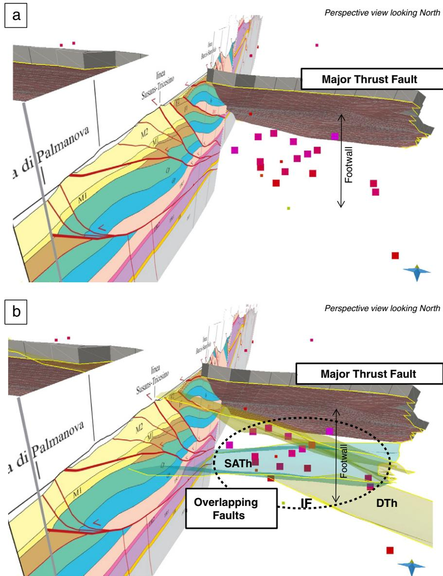
**Fig. 11.** 3D visualization of the Friuli domain seismo-tectonics:  $4 < M < 7$  earthquakes against 3D fault surfaces; a) earthquakes in the footwall of major thrust plane, perspective view looking NW; b) same earthquake cluster in panel a) at the Southern Alps–Dinarides structural interference (IF = interference zone; SATH = Southern Alps thrust; DTh = Dinaric thrust; see text for discussion). Perspective view looking NW.
