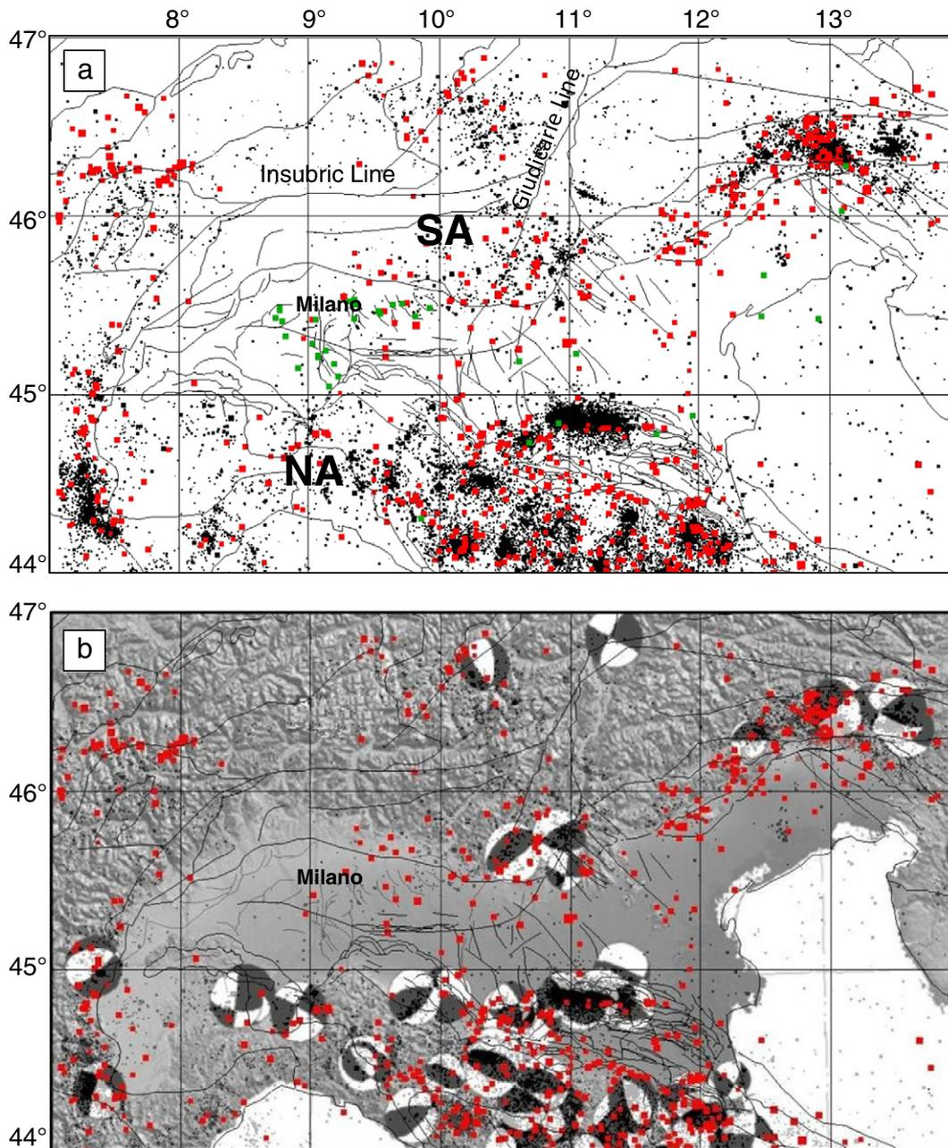
**Fig. 2.** a–b—Instrumental (black) and historical (red) earthquakes ( $0 < M < 7$ ) against the Po Valley tectonics (see Fig. 1 for unit distribution and name). Green squares in panel a are deep wells which have penetrated the Mesozoic Carbonates. In panel b the focal mechanisms of the major events ( $M > 5$ ; from Di Bucci and Angeloni, 2013) are indicated.
