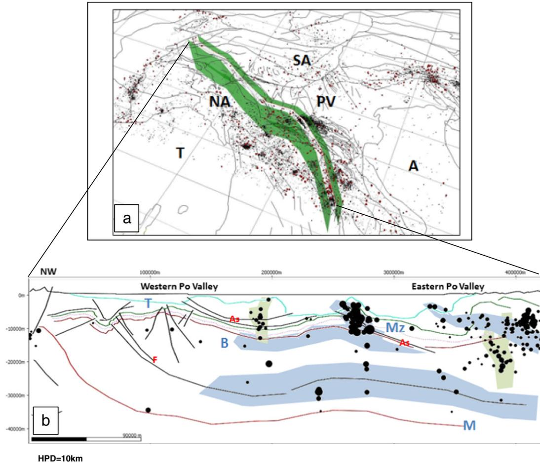
**Fig. 16.** Crustal section across the Po Valley and main seismogenic zones (light blue shadows). T: Tertiary sediments; Mz: Mesozoic sediments; B: basement; M: Moho. HPD = Hypocentre Projection Distance; v:h = 2.5:1.
