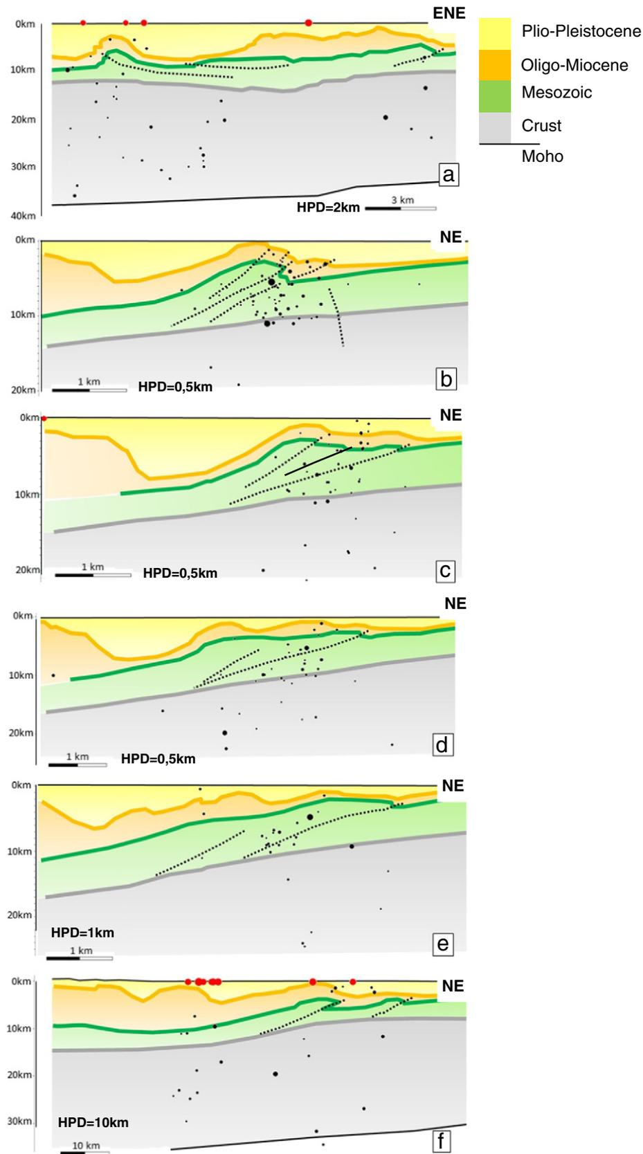
**Fig. 12.** Seismo-tectonic sections sliced across the 3D volume (location in Fig. 9b) to show structure–earthquake association across the Ferrara tectonic arc; HPD = Hypocentre Projection Distance; see text for discussion.
